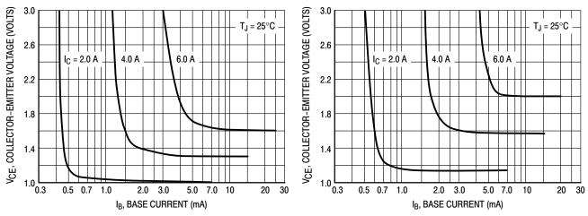
**Figure 6. Collector Saturation Region**
