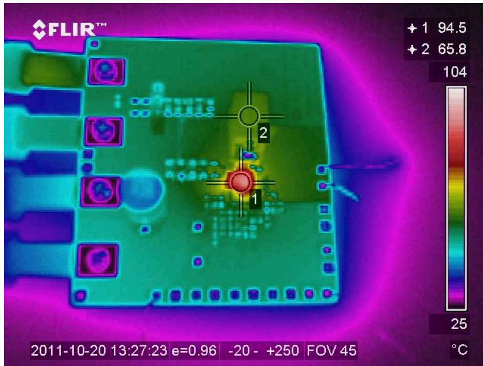
Figure 46: Thermal Image of the Board at 16A Load, Test Point 1 is IR3895, Test Point 2 is inductor
