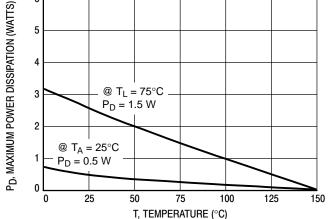
Figure 2. Pulse Derating Curve
