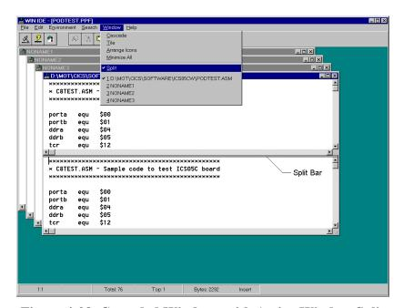
Figure 4-28. Cascaded Windows with Active Window Split
