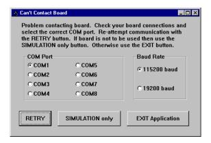
Figure 6-1. Can't Contact Board Dialog
