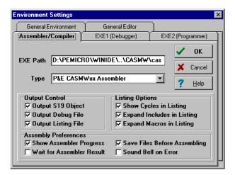
Figure 4-15. Environment Settings Dialog: Assembler/Compiler Tab
