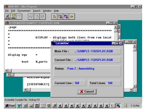
Figure 5-1. WinIDE with CASM05W Assembler Window Displayed
