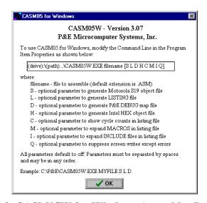
Figure 5-3. CASM05W for Windows Assembler Parameters
