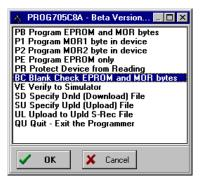
Figure 6-21. PROG05C Programmer Pick Window
