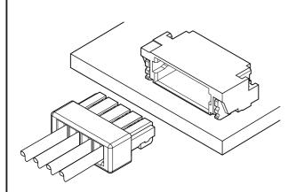
This SUH connector is developed for crimping type SUR connector that has been designed for 0.8 mm pitch wire-to-board insulation displacement connector. This connector adopted the first crimping method in a minimum 0.8 mm pitch of the wire-to-board type connector. Housing lance method provides the good workability and a constriction contact method provides the excellent contact reliability.
