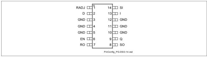
Figure 2 Pin Configuration (top view)
