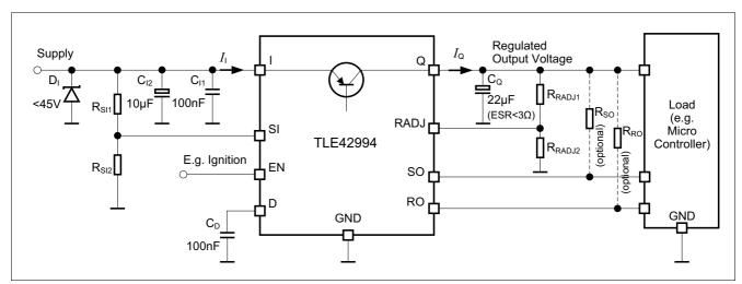
Figure 9 Application Diagram with Reset Thresholds Adjustment
