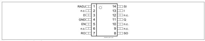
Figure 3 Pin Configuration (top view)
