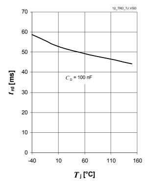
Delay Capacitor Discharge Time  $t_{\rm rr,d}$  versus Junction Temperature  $T_{\rm j}$
