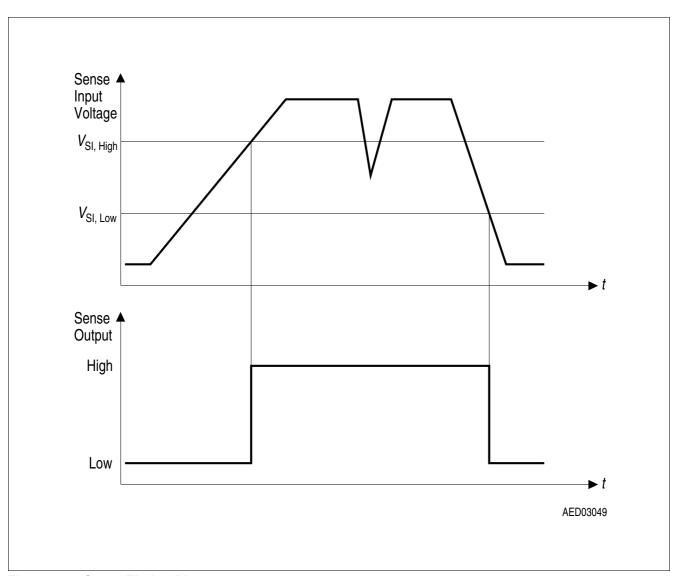
Figure 7 Sense Timing Diagram
