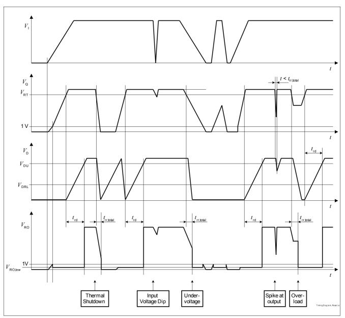
Figure 6 Timing Diagram Reset
