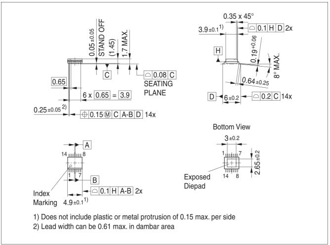
Figure 11 PG-SSOP-14 Exposed Pad
