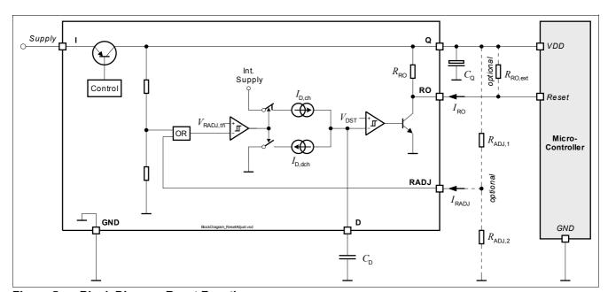
Figure 5 Block Diagram Reset Function
