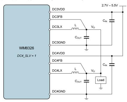
Figure 30 DC-DC3 / DC-DC4 Dual Mode Converter Connections
