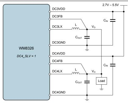
Figure 21 DC-DC3 / DC-DC4 Dual Mode Converter Connections
