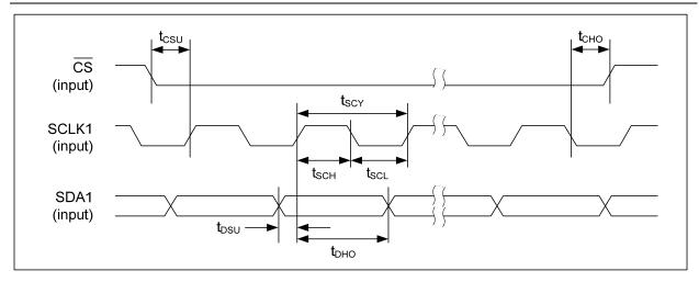
Figure 2 Control Interface Timing - 4-wire (SPI) Control Mode (Write Cycle)
