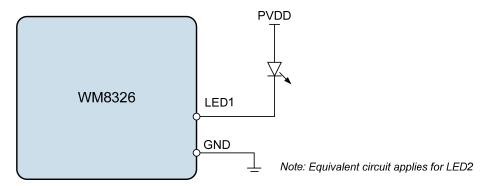
Figure 23 System Status LED Connections
