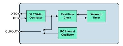
Figure 16 Clocking Configuration
