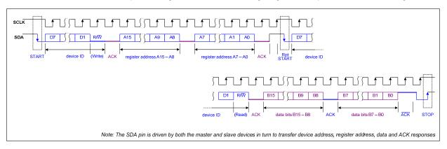
Figure 8 Control Interface 2-wire (I2C) Register Read
