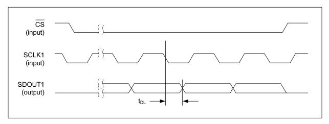
Figure 3 Control Interface Timing - 4-wire (SPI) Control Mode (Read Cycle)
