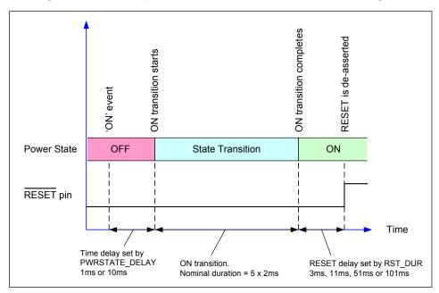
Figure 6 RESET Pin Output
