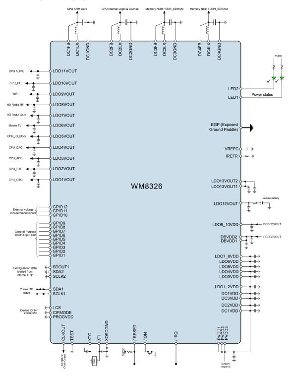
Figure 28 WM8326 Typical Connections Diagram
