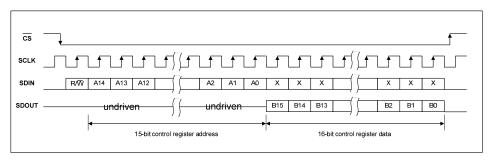
Figure 15 Control Interface 4-wire (SPI) Register Read
