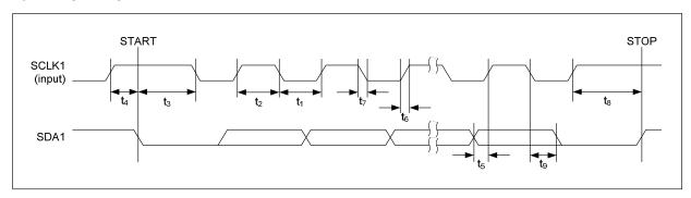
Figure 1 Control Interface Timing - 2-wire (I2C) Control Mode
