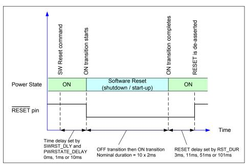
Figure 25 Software Reset Timing
