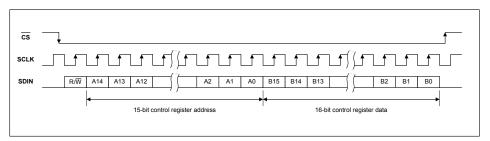
Figure 14 Control Interface 4-wire (SPI) Register Write
