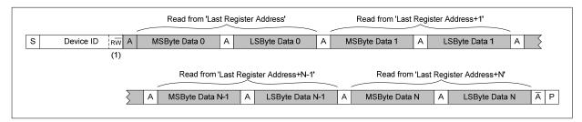
Figure 13 Multiple Register Read from Last Address using Auto-increment
