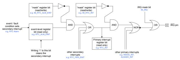
Figure 24 Interrupt Logic
