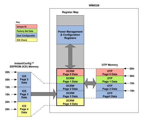
Note that the recommended external ICE memory is arranged in 8-bit words
