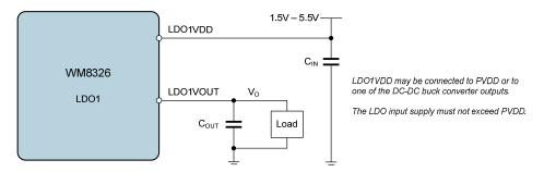
Note: Equivalent circuit applies for LDO2 through to LDO10.
