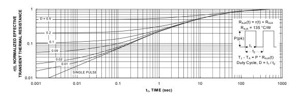
Figure 11. Transient Thermal Response Curve.
