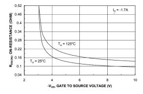
Figure 4. On-Resistance Variation with Gate-to-Source Voltage.
