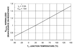
Figure 3. On-Resistance Variation with Temperature.
