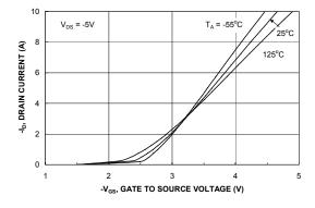
Figure 5. Transfer Characteristics.
