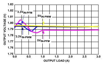
FIGURE 11. V<sub>OUT</sub> REGULATION vs LOAD (1MHz, V<sub>OUT</sub> = 1.8V)
