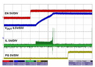
FIGURE 25. SOFT-START WITH PREBIASED 1V
