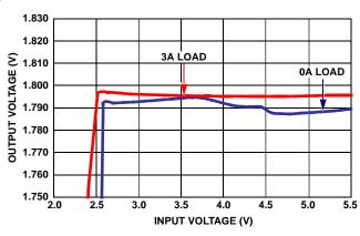
FIGURE 15. OUTPUT VOLTAGE REGULATION vs VIN (PFM V<sub>OUT</sub> = 1.8V)
