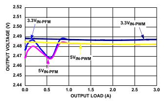
FIGURE 12. V<sub>OUT</sub> REGULATION vs LOAD (1MHz, V<sub>OUT</sub> = 2.5V)
