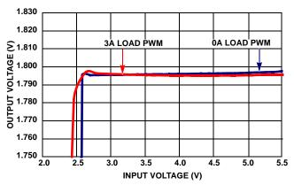
FIGURE 14. OUTPUT VOLTAGE REGULATION vs VIN (PWM  $V_{OUT} = 1.8$ )
