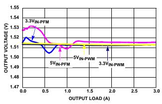
FIGURE 10.  $V_{OUT}$  REGULATION vs LOAD (1MHz,  $V_{OUT} = 1.5V$ )
