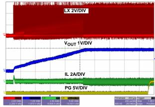
FIGURE 33. OUTPUT SHORT-CIRCUIT RECOVERY
