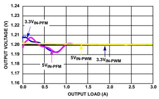
FIGURE 9. V<sub>OUT</sub> REGULATION vs LOAD (1MHz, V<sub>OUT</sub> = 1.2V)
