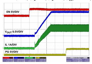
FIGURE 26. SOFT-START AT FULL LOAD
