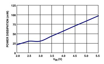
FIGURE 8. POWER DISSIPATION WITH NO LOAD vs  $V_{IN}$  (PWM  $V_{OUT}$  = 1.8V)
