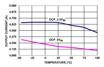
FIGURE 34. OUTPUT CURRENT LIMIT vs TEMPERATURE
