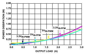
FIGURE 7. POWER DISSIPATION vs LOAD (1MHz, V<sub>OUT</sub> = 1.8V)
