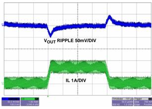
FIGURE 21. LOAD TRANSIENT (PWM)
