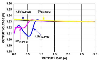
FIGURE 13. V<sub>OUT</sub> REGULATION vs LOAD (1MHz, V<sub>OUT</sub> = 3.3V)
