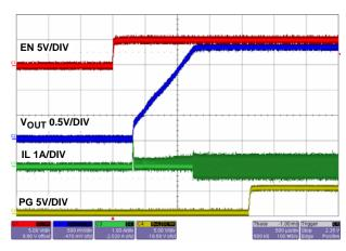
FIGURE 23. SOFT-START WITH NO LOAD (PWM)
