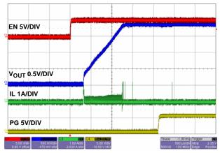
FIGURE 24. SOFT-START AT NO LOAD (PFM)
