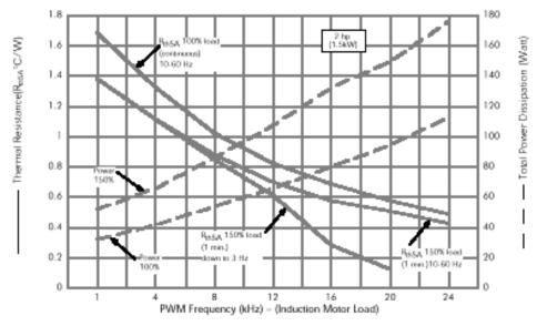
Figure 4b. 2 hp/4.2A Output Heat Sink Thermal Resistance and Power Dissipation vs. PWM Frequency NOTE: For figures 4a and 4b: Operating Conditions: V<sub>c1</sub> = 460V<sub>c10</sub>, MI = 1.15, PF = 0.8, T<sub>A</sub> = 40°C, T<sub>1</sub> < 145°C, T<sub>2</sub> < 95°C, Z<sub>60A</sub> limits ΔT<sub>c</sub> during 1 minute overload to 10°C
