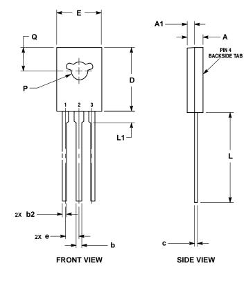
NOTES: 1. DIMENSIONING AND TOLERANCING PER ASME Y14.5M, 1994. 2. CONTROLLING DIMENSION: MILLIMETERS.
