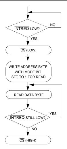
Figure 20. SPI Read Flow Diagram
