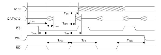
Figure 3. Intel<sup>®</sup> Parallel Host Mode Read Cycle
