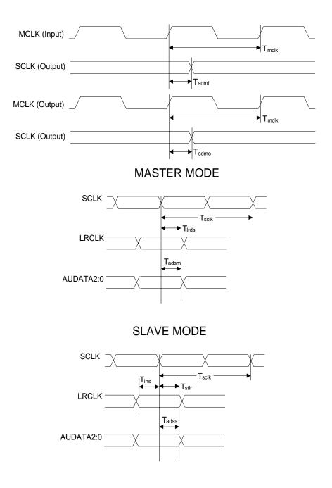
Figure 12. Digital Audio Output Data, Input and Output Clock Timing
