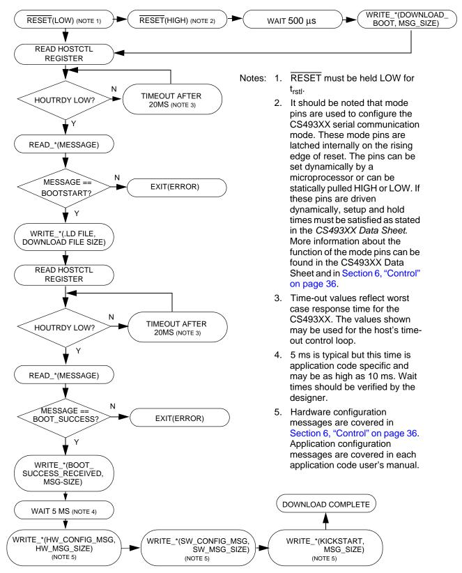
Figure 34. Typical Parallel Boot and Download Procedure
