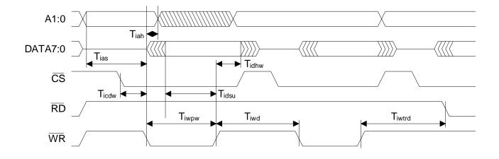
Figure 4. Intel<sup>®</sup> Parallel Host Mode Write Cycle
