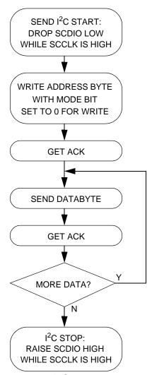
Figure 22. I<sup>2</sup>C<sup>®</sup> Write Flow Diagram
