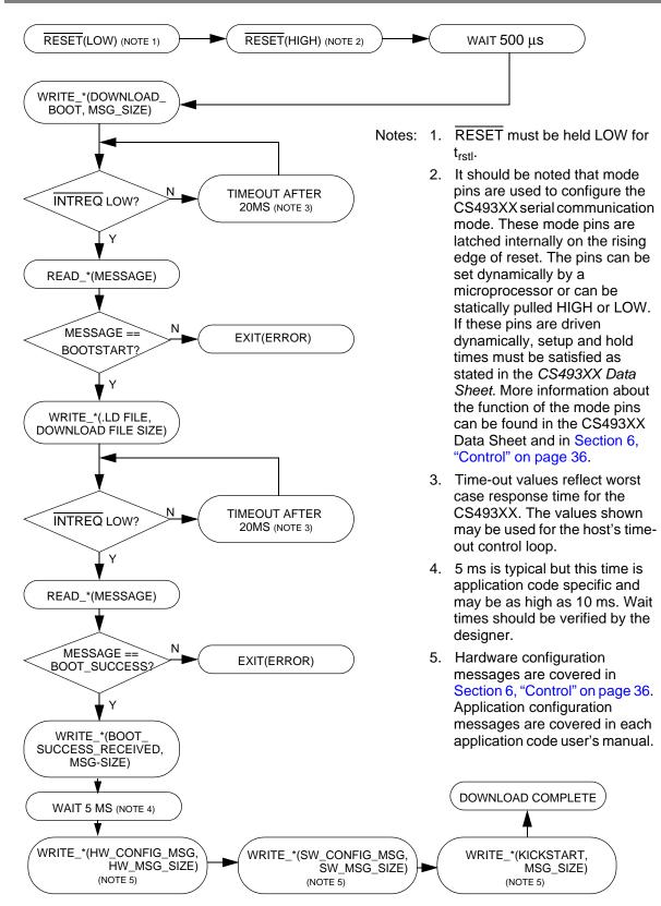
Figure 33. Typical Serial Boot and Download Procedure
