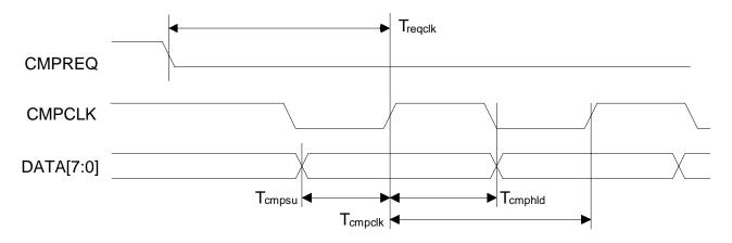
Figure 11. Parallel Data Timing (when not in a parallel control mode)
