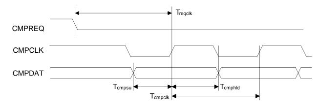
Figure 10. Serial Compressed Data Timing
