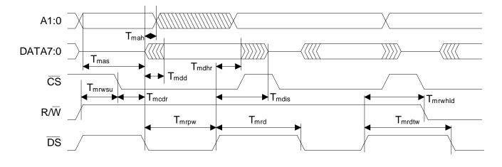
Figure 5. Motorola<sup>®</sup> Parallel Host Mode Read Cycle
