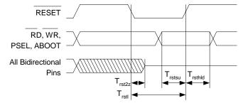
Figure 1. RESET Timing
