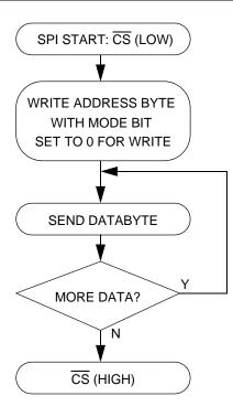
Figure 19. SPI Write Flow Diagram
