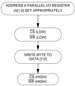
Figure 24. Intel Mode, One-Byte Write Flow Dia-
