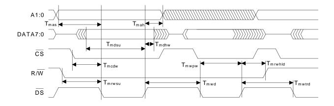
Figure 6. Motorola<sup>®</sup> Parallel Host Mode Write Cycle
