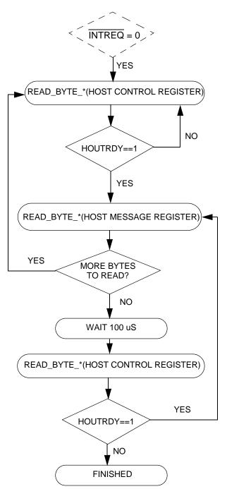
Figure 29. Typical Parallel Host Mode Control Read Sequence Flow Diagram
