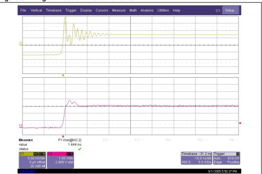
Figure 9. Digital crosstalk measurements
