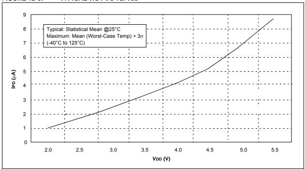
FIGURE 12-7: MAXIMUM WDT IPD vs. VDD OVER TEMPERATURE
