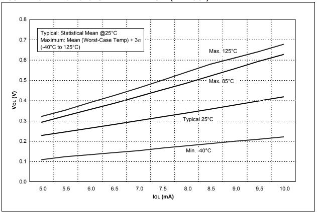
FIGURE 12-10: Vol vs. Iol OVER TEMPERATURE (VDD = 5.0V)
