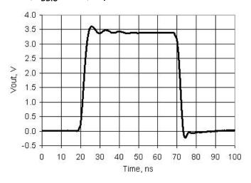
Figure 11-21. SIO Output Rise and Fall Times, Slow Strong Mode,  $V_{DDIO} = 3.3 \text{ V}$ , 25 pF Load
