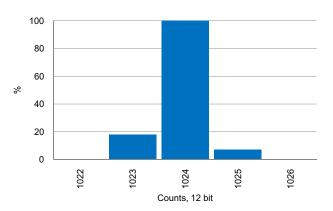
Figure 11-41. SAR ADC Noise Histogram, 1 msps, External Reference
