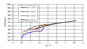
Figure 11-13. Efficiency vs  $V_{BAT}$ ,  $L_{BOOST}$  = 22  $\mu H^{[33]}$
