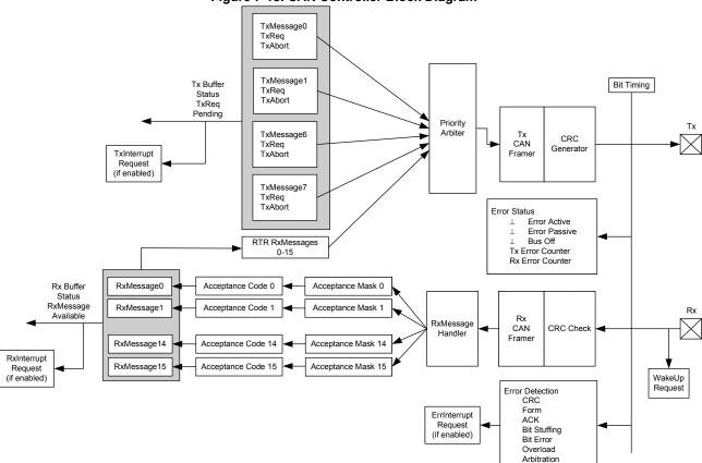
Figure 7-15. CAN Controller Block Diagram
