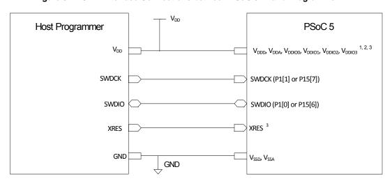
Figure 9-2. SWD Interface Connections between PSoC 5LP and Programmer
