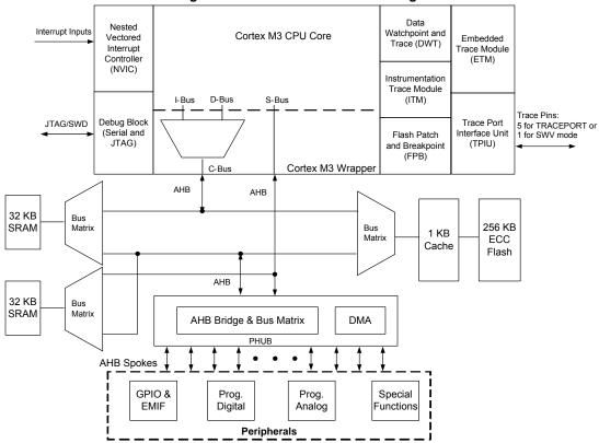
Figure 4-1. ARM Cortex-M3 Block Diagram
