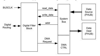
The typical use model is for data to be supplied to the DFB over the system bus from another on-chip system data source such as an ADC. The data typically passes through main memory or is directly transferred from another chip resource through DMA. The DFB processes this data and passes the result to another on chip resource such as a DAC or main memory through DMA on the system bus.
