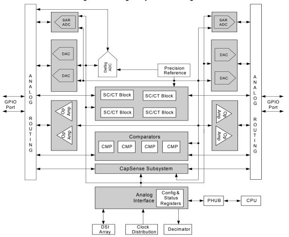
Figure 8-1. Analog Subsystem Block Diagram
