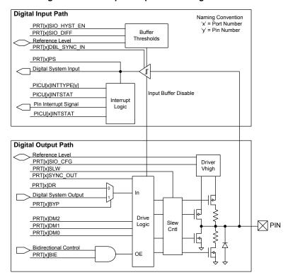
Figure 6-10. SIO Input/Output Block Diagram
