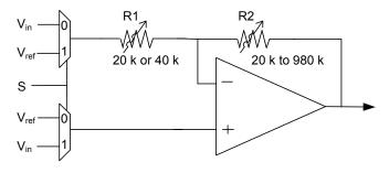
The PGA is used in applications where the input signal may not be large enough to achieve the desired resolution in the ADC, or dynamic range of another SC/CT block such as a mixer. The gain is adjustable at runtime, including changing the gain of the PGA prior to each ADC sample.
