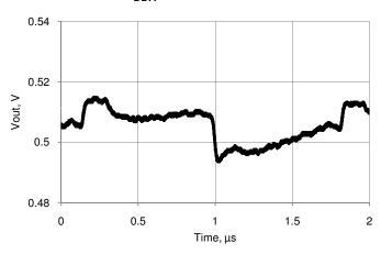
Figure 11-67. VDAC Voltage Noise, 1 V Mode, Fast Mode,  $V_{DDA} = 5 \text{ V}$
