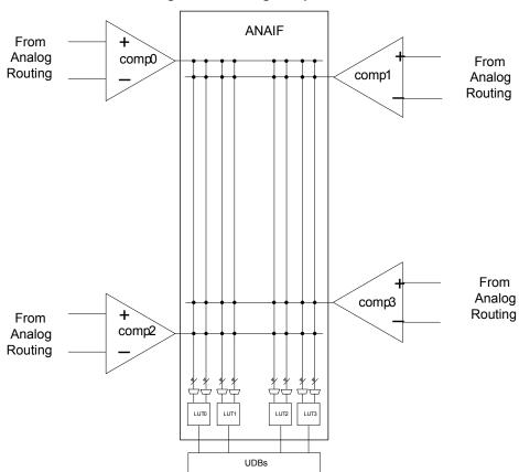
Figure 8-6. Analog Comparator
