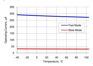
Figure 11-51. IDAC Operating Current vs Temperature, Range = 255 μA, Code = 0, Sink Mode
