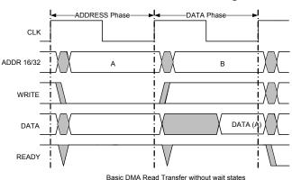
Figure 4-2. DMA Timing Diagram
