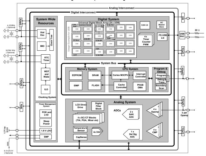
Figure 1-1. Simplified Block Diagram
