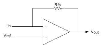
The TIA configuration is used for applications where an external sensor's output is current as a function of some type of stimulus such as temperature, light, magnetic flux etc. In a common application, the voltage DAC output can be connected to the  $V_{REF}$  TIA input to allow calibration of the external sensor bias current by adjusting the voltage DAC output voltage.
