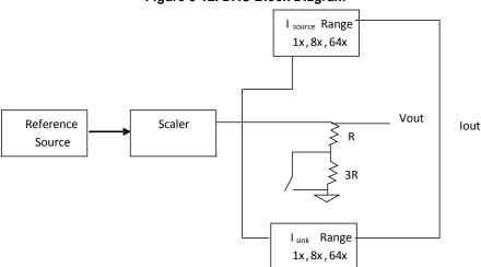
Figure 8-12. DAC Block Diagram
