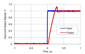
Figure 11-32. Opamp Step Response, Falling
