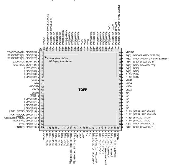
Figure 2-4. 100-pin TQFP Part Pinout
