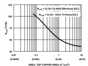
Figure 21. Thermal Resistance vs Mounting Pad Area
