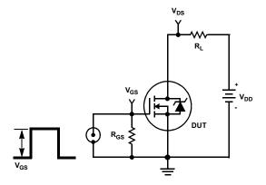
Figure 19. Switching Time Test Circuit
