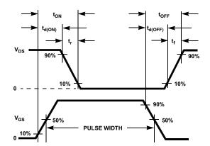
Figure 20. Switching Time Waveforms
