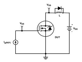
Figure 17. Gate Charge Test Circuit
