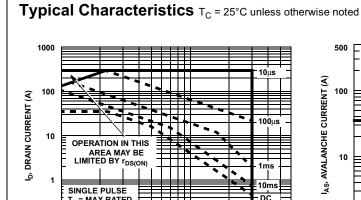
If R = 0  $t_{AV} = (L)(I_{AS})/(1.3*RATED BV_{DSS})$ IAS, AVALANCHE CURRENT (A) STARTING T<sub>J</sub> = 25°C 10 0.01 t<sub>AV</sub>, TIME IN AVALANCHE (ms)
