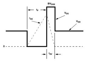
Figure 16. Unclamped Energy Waveforms
