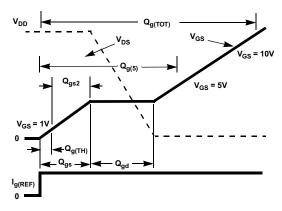
Figure 18. Gate Charge Waveforms
