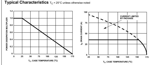
Figure 1. Normalized Power Dissipation vs Case Temperature
