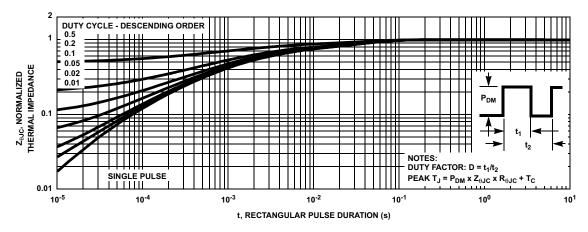
Figure 3. Normalized Maximum Transient Thermal Impedance
