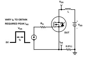
Figure 15. Unclamped Energy Test Circuit
