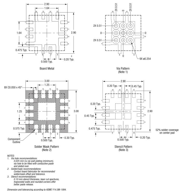
Unless specified, dimensions are symmetrical about center lines. All dimensions are in millimeters.
