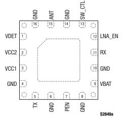
Figure 2. SKY85709-11 Pinout – 16-Pin QFN (Top View)
