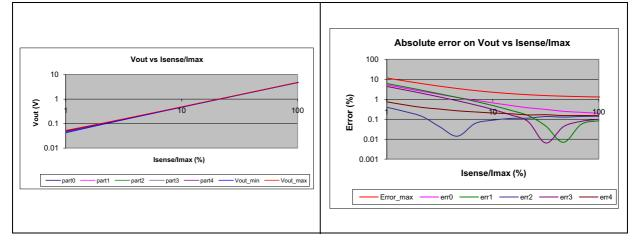
Figure 9. Case 4: Rshunt = 100 m $\Omega$ , Rg = 100  $\Omega$ , Rf = 4.75 k $\Omega$ , Imax = 1 A
