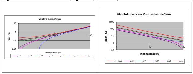
Figure 7. Case 2: Rshunt = 10 m $\Omega$ , Rg = 100  $\Omega$ , Rf = 47.5 k $\Omega$ , Imax = 1 A
