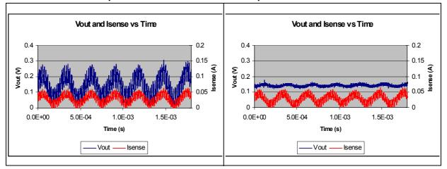
As you can see, the signal is filtered. If you increased the capacitor to 1  $\mu$ F instead of 100 nF you would obtain an even smoother response.
