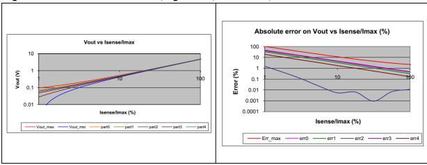
Figure 8. Case 3: Rshunt = 30 m $\Omega$ , Rg = 100  $\Omega$ , Rf = 16.2 k $\Omega$ , Imax = 1 A
