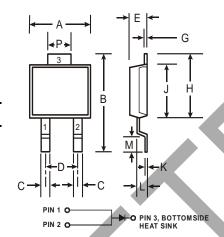
POWERMITE®3 Dim Min Max 4.03 4.09 Α В 6.40 6.61 .889 NOM C D 1.83 NOM Ε 1.10 1.14 G .178 NOM 5.01 5.17 J 4.37 4.43 K .178 NOM L .71 .77 М .36 .46 P 1.73 1.83 All Dimensions in mm
