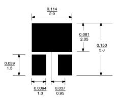
FIGURE 1. Footprint With Copper Spreading
