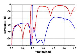
Figure 10. Tx–Ant and Ant–Rx wideband insertion loss
