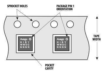
Figure 21. Unit orientation In tape
