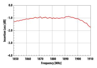
Figure 3. Tx–Ant insertion loss
