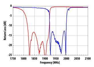
Figure 5. Tx and Rx port return loss
