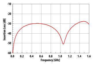
Figure 11. Tx–Ant low frequency rejection
