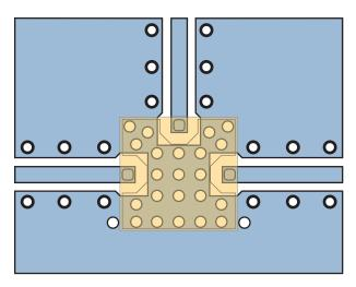
Figure 16. Duplexer superposed on PCB land print
