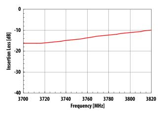
Figure 9. Tx–Ant rejection at Tx second harmonic
