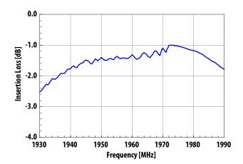
Figure 4. Ant–Rx insertion loss
