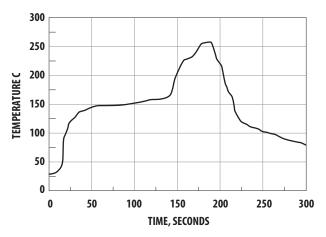
Figure 19. Verified SMT solder profile
