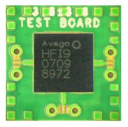
Figure 2. Test circuit with ACMD-7409 duplexer
