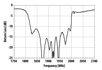
Figure 8. Antenna port return loss
