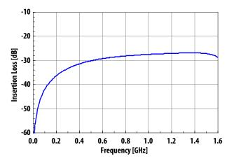
Figure 12. Ant-Rx low frequency rejection
