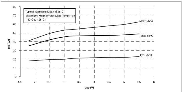
FIGURE 24-14: PIC16LF720/721 MAXIMUM BASE IPD vs. VDD
