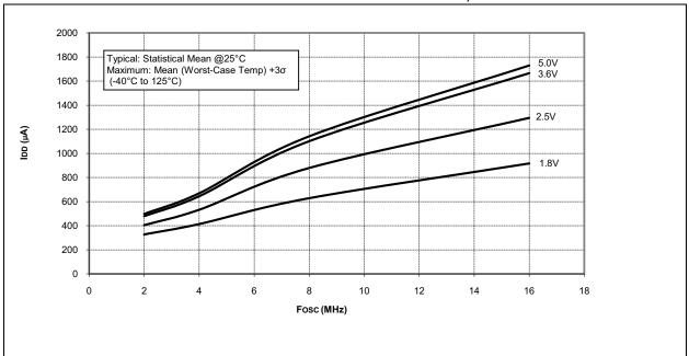
FIGURE 24-11: PIC16LF720/721 MAX. IDD vs. Fosc OVER VDD, HFINTOSC
