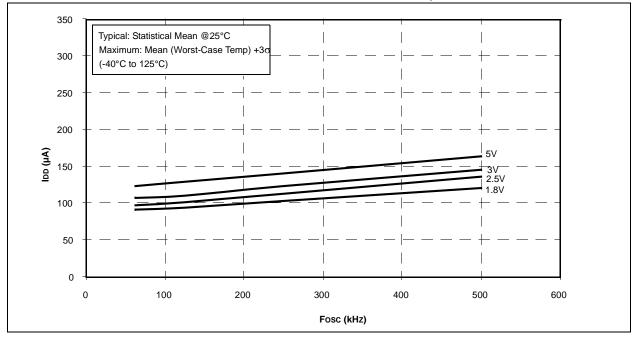
FIGURE 24-7: PIC16LF720/721 MAX. IDD vs. Fosc OVER VDD, MFINTOSC
