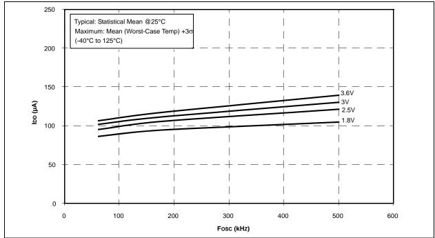
FIGURE 24-9: PIC16F720/721 MAX. IDD vs. Fosc OVER VDD, HFINTOSC
