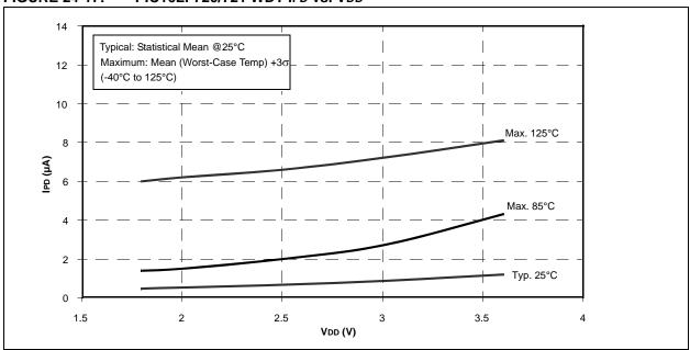
FIGURE 24-18: PIC16F720/721 FIXED VOLTAGE REFERENCE IPD vs. VDD
