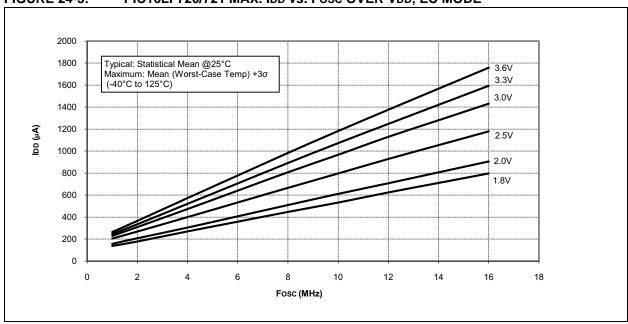
FIGURE 24-4: PIC16LF720/721 TYPICAL IDD vs. Fosc OVER VDD, EC MODE
