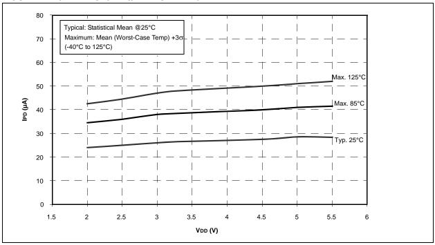
FIGURE 24-21: PIC16LF720/721 BOR IPD vs. VDD
