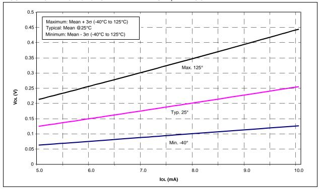
FIGURE 24-29: Vol vs. Iol OVER TEMPERATURE, VDD = 3.6
