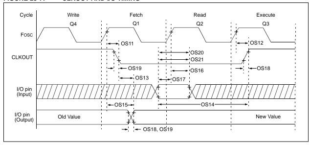
TABLE 23-3: CLKOUT AND I/O TIMING PARAMETERS
