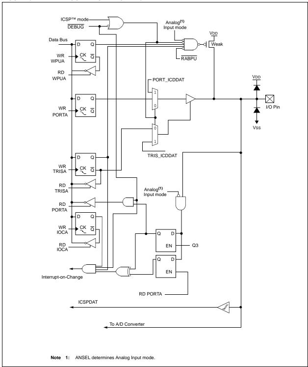
FIGURE 6-2: **BLOCK DIAGRAM OF RA1** ICSP™ mode Analog<sup>(1)</sup> Input mode Data Bus DEBUG -V<sub>DD</sub> WR WPUA Q Weak RABPU RD WPUA Q PORT\_ICDCLK Q WR PORTA Q WR TRISA RD TRISA Analog<sup>(1)</sup> Input mode TRIS\_ICDCLK RD PORTA Q D Q WR IOCA ΕN RD IOCA D Interrupt-on-Change ΕN RD PORTA -To A/D Converter **ICSPCLK** Note 1: ANSEL determines Analog Input mode.
