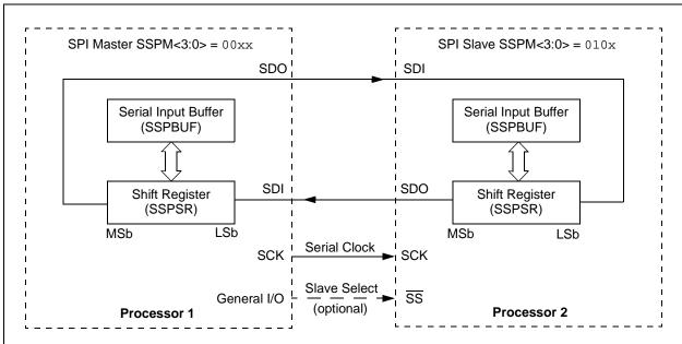
FIGURE 17-2: SPI MODE BLOCK DIAGRAM
