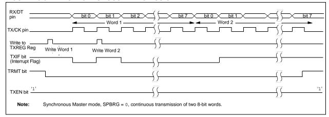
FIGURE 16-7: SYNCHRONOUS TRANSMISSION (THROUGH TXEN)
