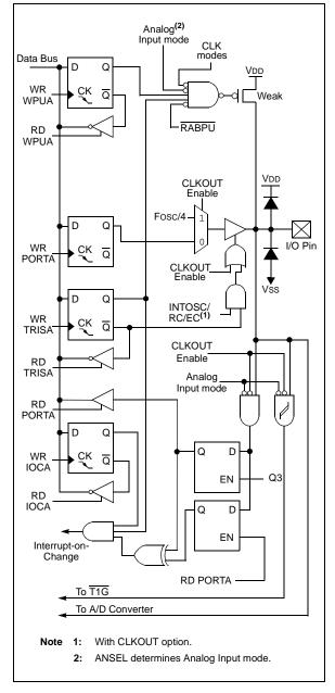
FIGURE 6-6: BLOCK DIAGRAM OF RA5
