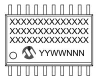
20-Lead SSOP (5.30 mm)
