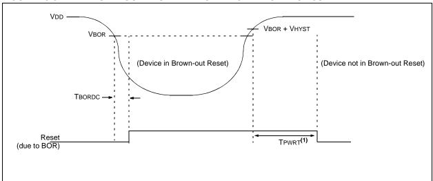
TABLE 23-4: RESET, WATCHDOG TIME, POWER-UP TIMER, AND BROWN-OUT RESET PARAMETERS
