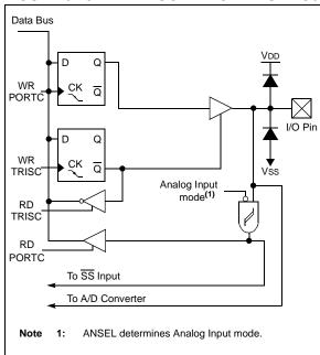
FIGURE 6-16: BLOCK DIAGRAM OF RC7
