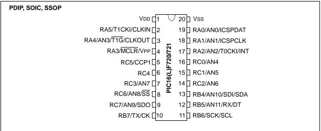
Pin Diagrams - 20-PIN DIAGRAM FOR PIC16(L)F720/721
