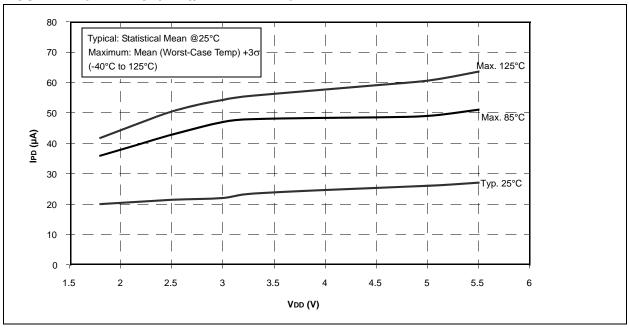
FIGURE 24-17: PIC16LF720/721 WDT IPD vs. VDD
