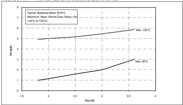
FIGURE 24-15: PIC16LF720/721 TYPICAL BASE IPD vs. VDD
