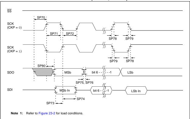
FIGURE 23-16: SPI MASTER MODE TIMING (CKE = 1, SMP = 1)
