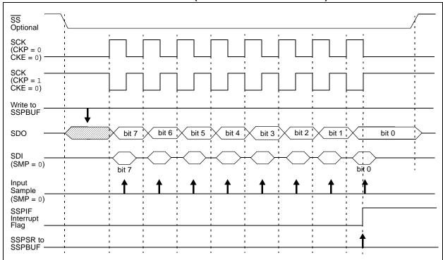
FIGURE 17-5: SPI MODE WAVEFORM (SLAVE MODE WITH CKE = 1)
