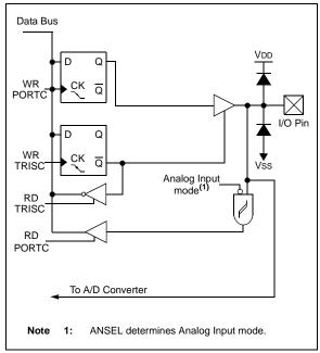
FIGURE 6-13: BLOCK DIAGRAM OF RC4
