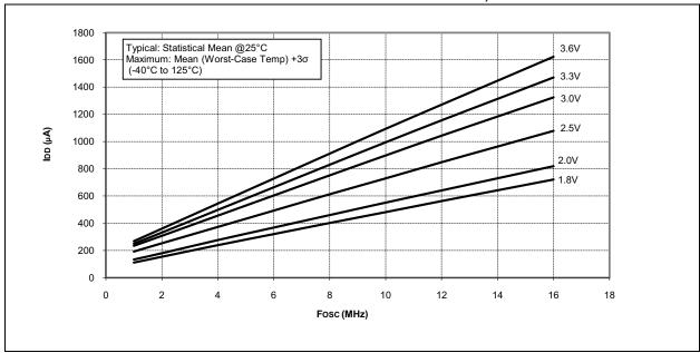
FIGURE 24-5: PIC16F720/721 MAX. IDD vs. Fosc OVER VDD, MFINTOSC
