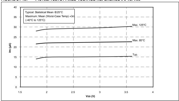
FIGURE 24-20: PIC16F720/721 BOR IPD vs. VDD
