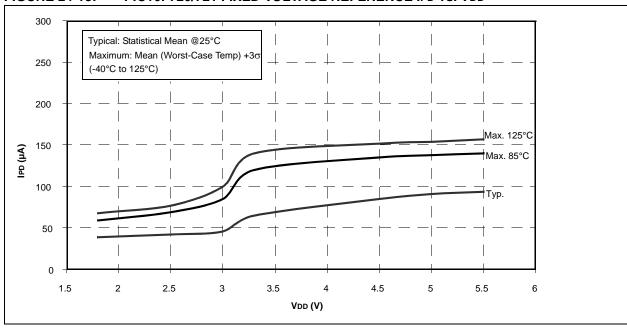
FIGURE 24-19: PIC16LF720/721 FIXED VOLTAGE REFERENCE IPD vs. VDD
