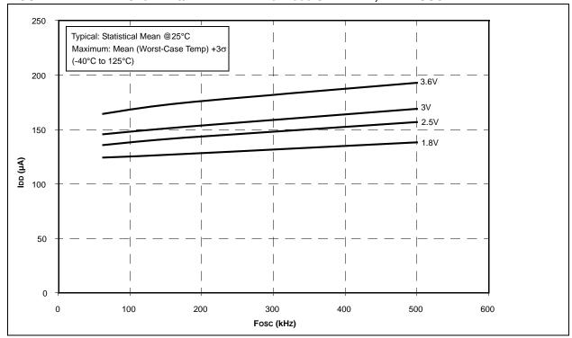
FIGURE 24-8: PIC16LF720/721 TYPICAL IDD vs. Fosc OVER VDD, MFINTOSC
