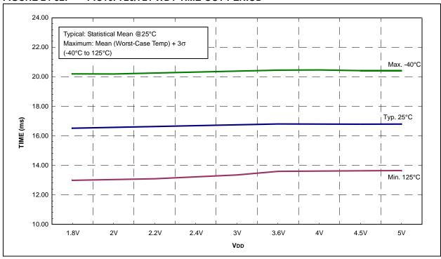
FIGURE 24-33: PIC16F720/721 HFINTOSC WAKE-UP FROM SLEEP START-UP TIME
