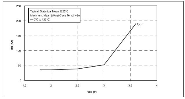
FIGURE 24-16: PIC16F720/721 WDT IPD vs. VDD
