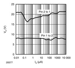
Fig. 4 - Typical Reverse Voltage  $V_{\text{R}}$  vs. Reverse Current  $I_{\text{R}}$
