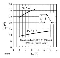
Fig. 5 - Typical Peak Clamping Voltage  $V_{\rm C}$  vs. Peak Pulse Current  $I_{\rm PP}$
