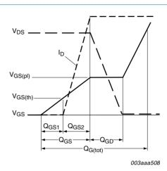
Fig 12. Gate charge waveform definitions
