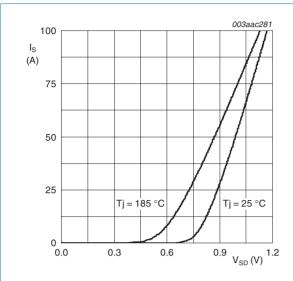
Fig 11. Source current as a function of source-drain voltage; typical values
