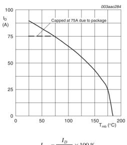
$$I_{der} = \frac{I_D}{I_{D(25^{\circ}C)}} \times 100 \%$$
