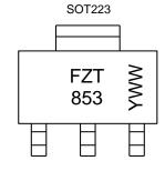
FZT 853 = Product Type Marking Code YWW = Date Code Marking Y or  $\overline{Y}$  = Last Digit of Year (ex: 5 = 2015) WW or  $\overline{W}W$  = Week Code (01–53)
