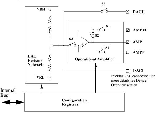
Figure 19-1. DAC\_8B5V Block Diagram
