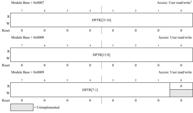
Figure 7-5. ECC Debug Pointer Register (ECCDPTRH, ECCDPTRM, ECCDPTRL)
