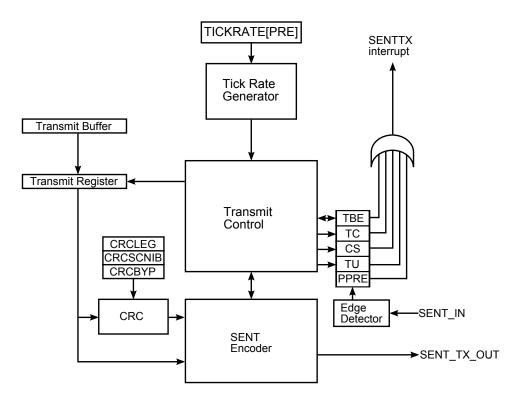
Figure 21-1. SENTTX Block Diagram
