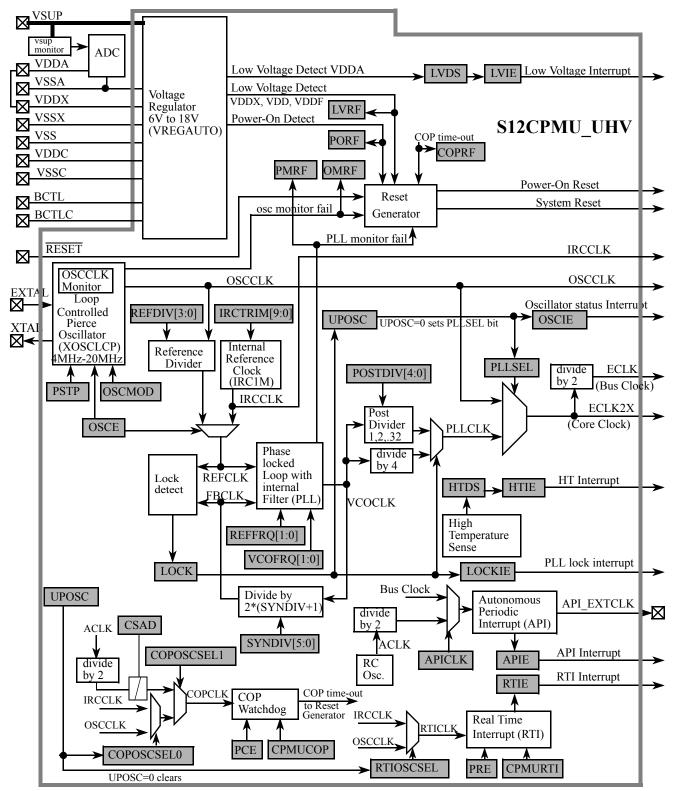
Figure 8-1. Block diagram of S12CPMU UHV V7
