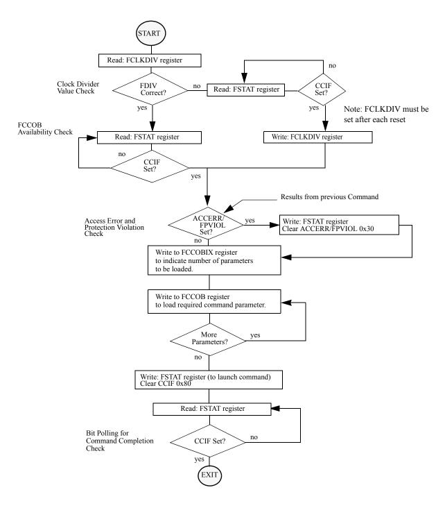
Figure 22-30. Generic Flash Command Write Sequence Flowchart
