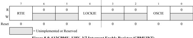
Figure 8-9. S12CPMU\_UHV\_V7 Interrupt Enable Register (CPMUINT)
