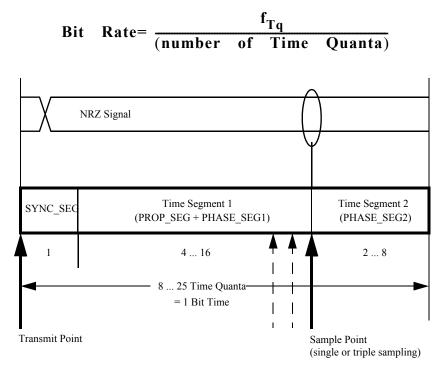
Figure 18-44. Segments within the Bit Time
