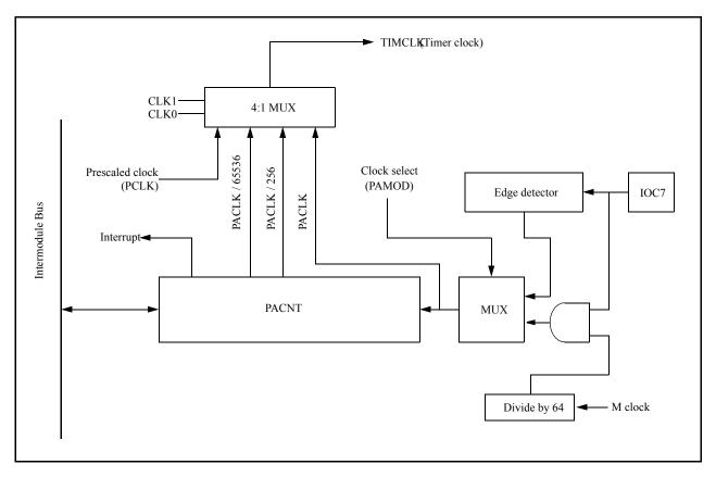
Figure 11-2. 16-Bit Pulse Accumulator Block Diagram
