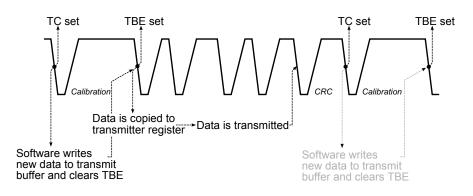
Figure 21-4. Transmission Complete driven SENT transfer without Pause Pulse
