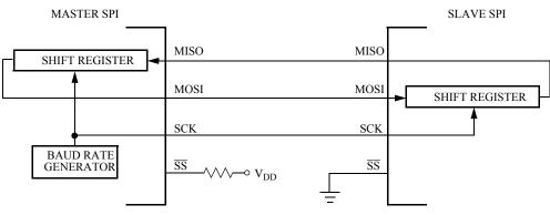
Figure 15-11. Master/Slave Transfer Block Diagram
