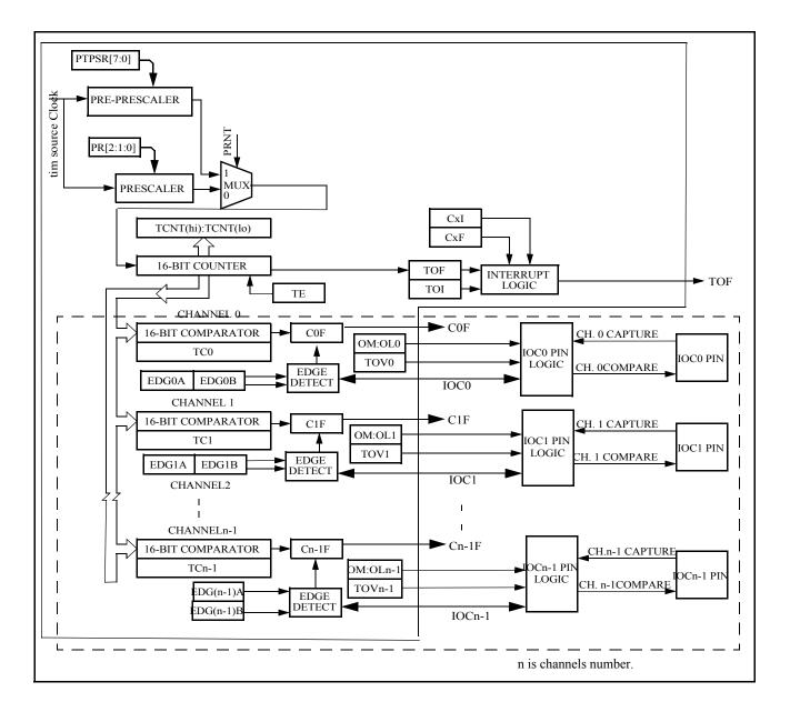
Figure 12-22. Detailed Timer Block Diagram
