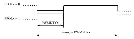
Figure 13-17. PWM Left Aligned Output Waveform
