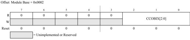
Figure 22-7. FCCOB Index Register (FCCOBIX)
