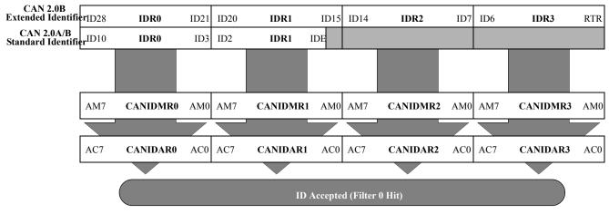
Figure 18-40. 32-bit Maskable Identifier Acceptance Filter
