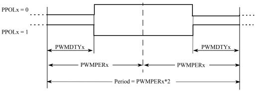
Figure 13-19. PWM Center Aligned Output Waveform
