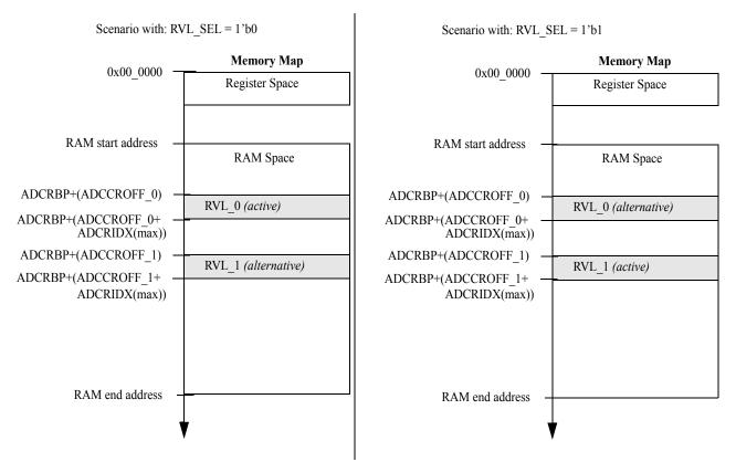
Note: Address register names in () are not absolute addresses instead they are a sample offset or sample index
