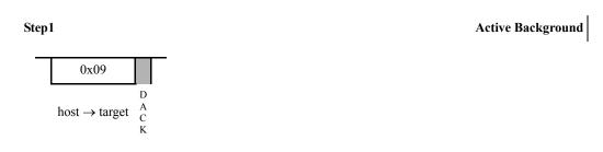
This command is used to step through application code. In active BDM this command executes the next CPU instruction in application code. If enabled an ACK is driven.
