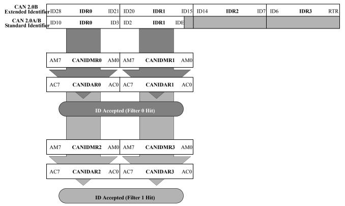
Figure 18-41. 16-bit Maskable Identifier Acceptance Filters
