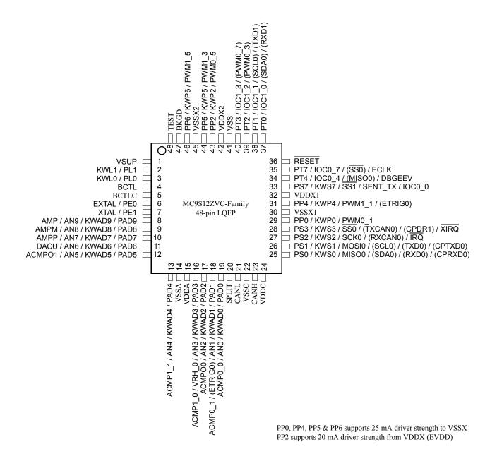
Figure 1-3. Pinout MC9S12ZVC-Family 48-pin LQFP
