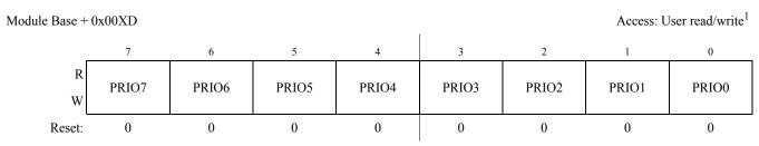
Figure 18-36. Transmit Buffer Priority Register (TBPR)
