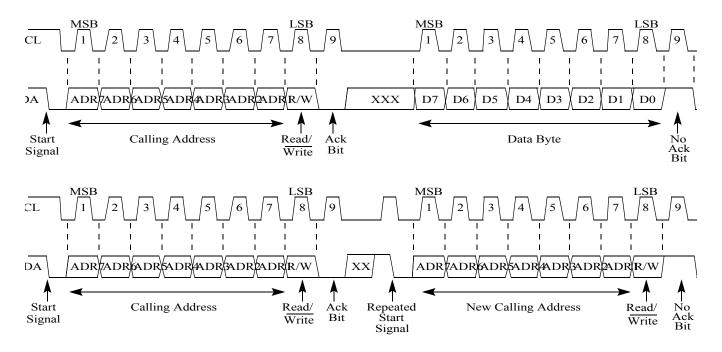
Figure 16-10. IIC-Bus Transmission Signals
