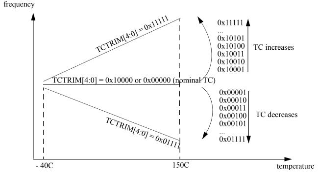
Figure 8-30. Influence of TCTRIM[4:0] on the Temperature Coefficient
