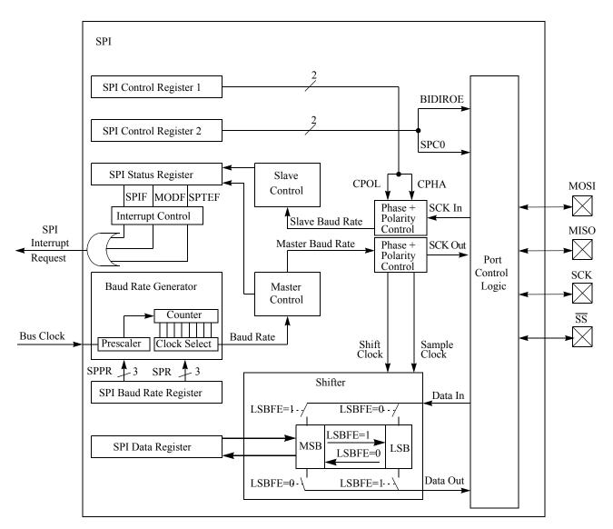
Figure 15-1. SPI Block Diagram
