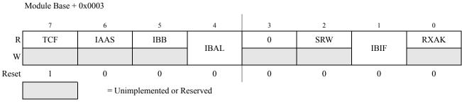
Figure 16-7. IIC Bus Status Register (IBSR)
