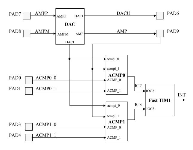
Figure 1-5. DAC , ACMP and Pad Connectivity
