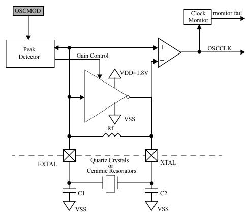
Figure 8-2. XOSCLCP Block Diagram
