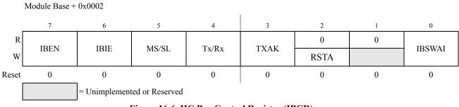
Figure 16-6. IIC Bus Control Register (IBCR)
