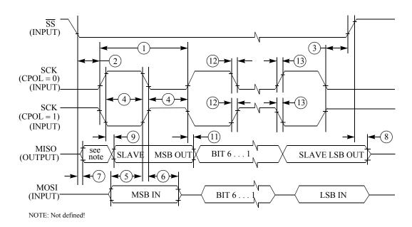
Figure D-5. SPI Slave Timing (CPHA=1)
