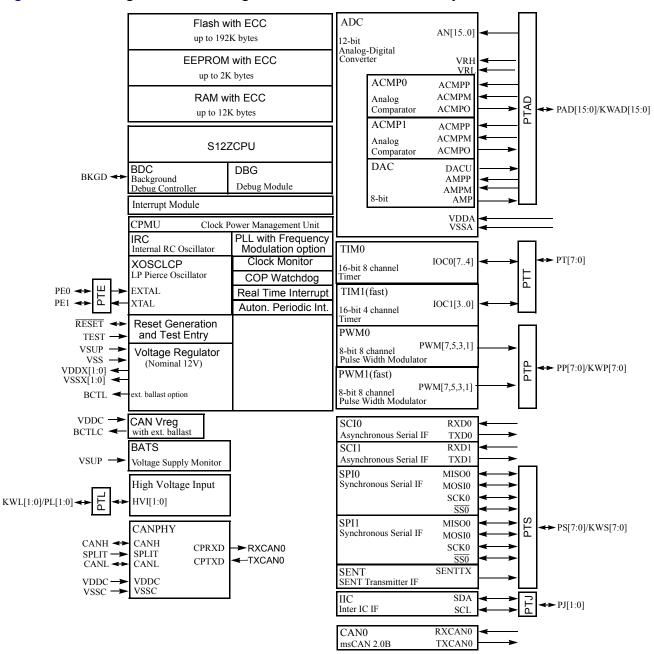
Block Diagram shows the maximum configuration! Not all pins or all peripherals are available on all devices and packages. Rerouting options are not shown.
