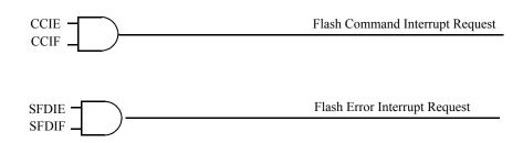
Figure 22-31. Flash Module Interrupts Implementation
