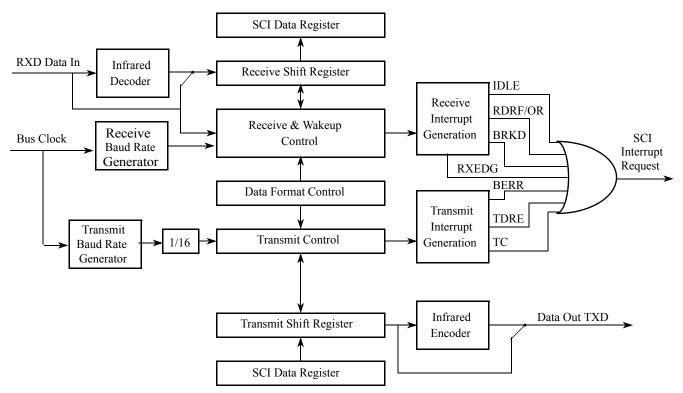
Figure 14-1. SCI Block Diagram
