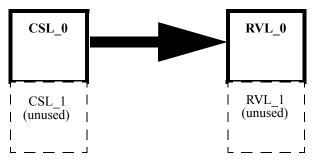
Figure 9-35. CSL Single Buffer Mode — RVL Single Buffer Mode Diagram
