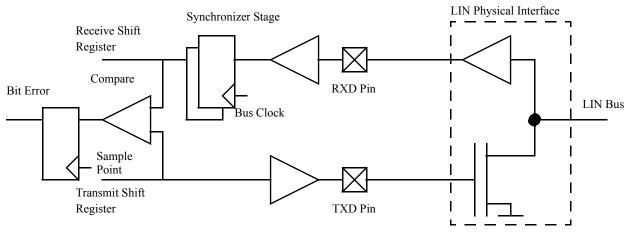
Figure 14-18. Collision Detect Principle
