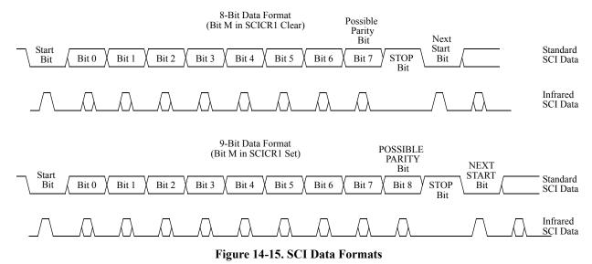
Each data character is contained in a frame that includes a start bit, eight or nine data bits, and a stop bit. Clearing the M bit in SCI control register 1 configures the SCI for 8-bit data characters. A frame with eight data bits has a total of 10 bits. Setting the M bit configures the SCI for nine-bit data characters. A frame
