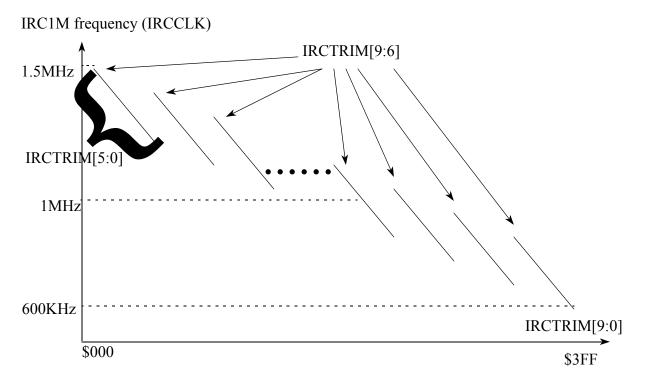
Figure 8-29. IRC1M Frequency Trimming Diagram
