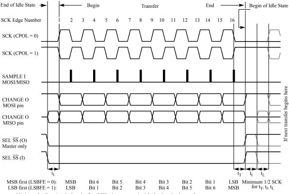
$t_L$  = Minimum leading time before the first SCK edge, not required for back-to-back transfers
