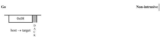
This command is used to exit active BDM and begin (or resume) execution of CPU application code. The CPU pipeline is flushed and refilled before normal instruction execution resumes. Prefetching begins at the current address in the PC. If any register (such as the PC) is altered by a BDC command whilst in BDM, the updated value is used when prefetching resumes. If enabled, an ACK is driven on exiting active BDM.
