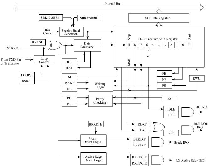
Figure 14-20. SCI Receiver Block Diagram
