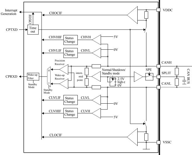
Figure 17-1. CAN Physical Layer Block Diagram
