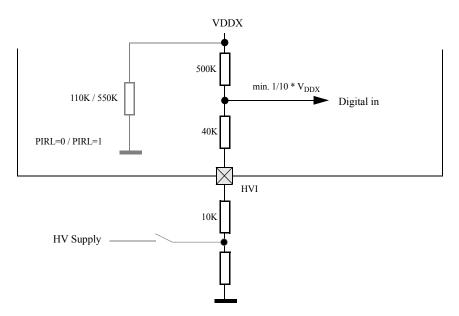
Figure 2-36. Digital Input Read with Pullup Enabled
