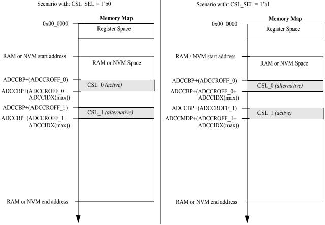
Note: Address register names in () are not absolute addresses instead they are a sample offset or sample index
