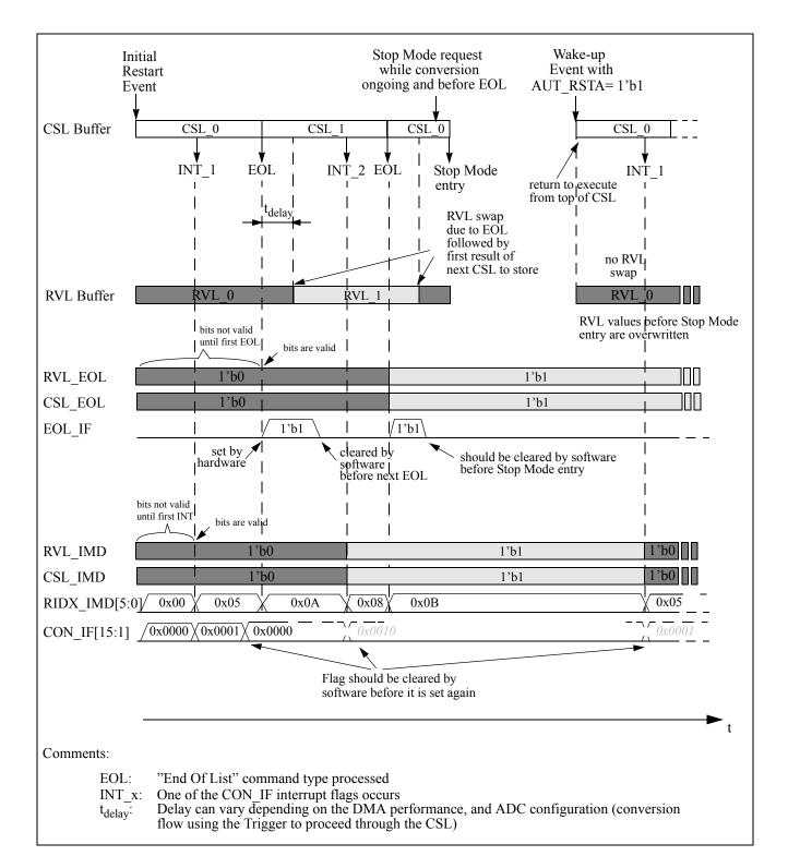
Figure 9-40. RVL Swapping — Use Case Diagram
