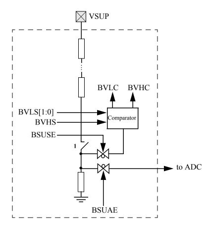
1 automatically closed if BSUSE and/or BSUAE is active, open during Stop mode
