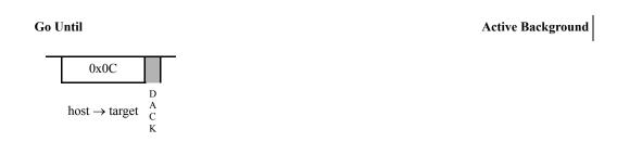
This command is used to exit active BDM and begin (or resume) execution of application code. The CPU pipeline is flushed and refilled before normal instruction execution resumes. Prefetching begins at the current address in the PC. If any register (such as the PC) is altered by a BDC command whilst in BDM, the updated value is used when prefetching resumes.
