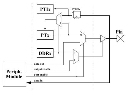
Figure 2-33. Illustration of I/O pin functionality
