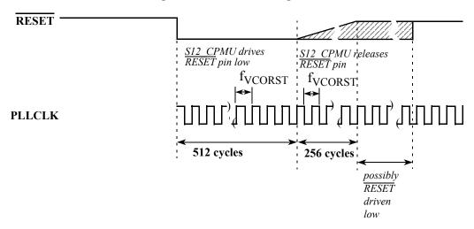
Figure 8-40. RESET Timing
