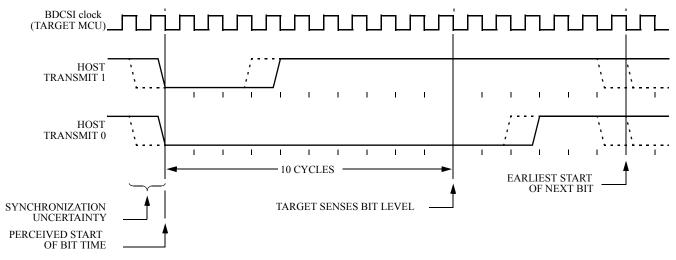
Figure 3-6. BDC Host-to-Target Serial Bit Timing
