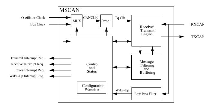
Figure 18-1. MSCAN Block Diagram
