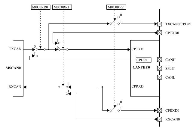
Figure 2-2. CAN Routing Options Illustration
