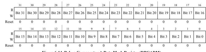
Figure 6-14. Debug Comparator A Data Mask Register (DBGADM)
