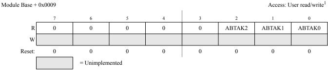
Figure 18-13. MSCAN Transmitter Message Abort Acknowledge Register (CANTAAK)
