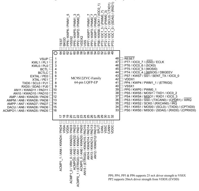
Figure 1-4. Pinout MC9S12ZVC-Family 64-pin LQFP-EP<sup>1</sup>
