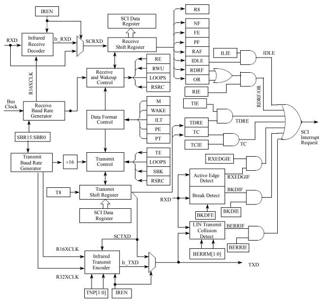
Figure 14-14. Detailed SCI Block Diagram
