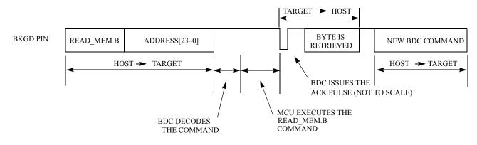
Figure 3-10. Handshake Protocol at Command Level
