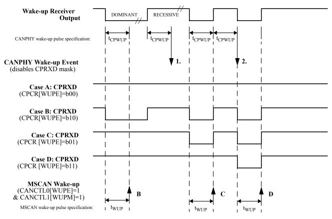
Figure 17-11. Wake-up Event Filtering
