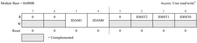
Figure 18-15. MSCAN Identifier Acceptance Control Register (CANIDAC)
