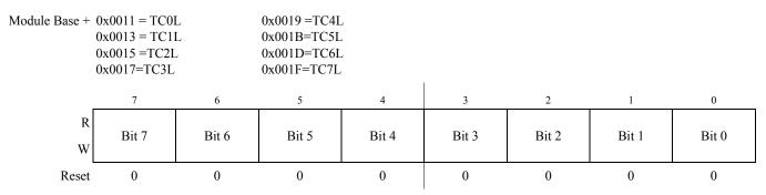
Figure 11-23. Timer Input Capture/Output Compare Register x Low (TCxL)
