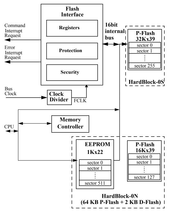
Figure 22-1. FTMRZ192K2K Block Diagram
