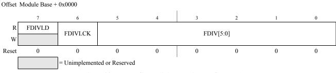
Figure 22-5. Flash Clock Divider Register (FCLKDIV)
