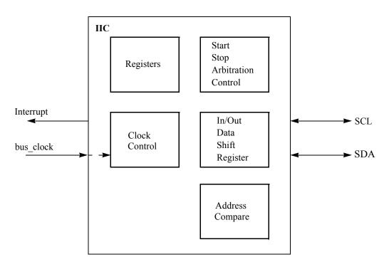
Figure 16-1. IIC Block Diagram
