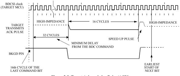
Figure 3-9. Target Acknowledge Pulse (ACK)
