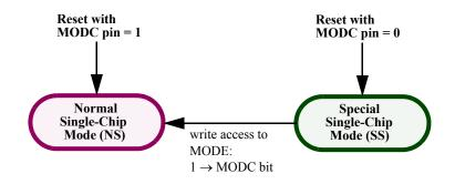
Figure 4-4. Mode Transition Diagram
