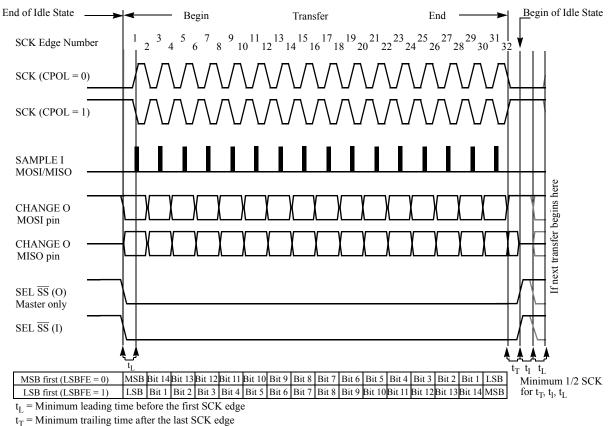
$t_{I}$  = Minimum idling time between transfers (minimum  $\overline{SS}$  high time)
