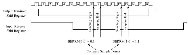
Figure 14-19. Timing Diagram Bit Error Detection
