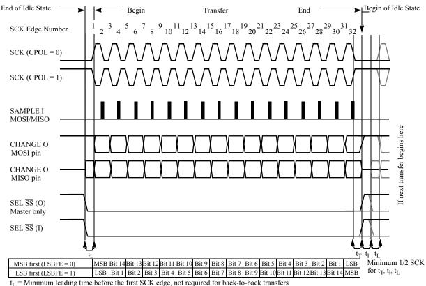
$t_{\rm T}$  = Minimum trailing time after the last SCK edge
