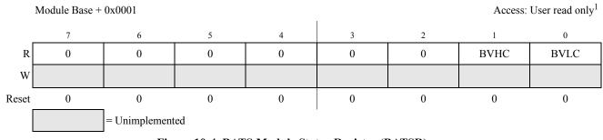
Figure 10-4. BATS Module Status Register (BATSR)
