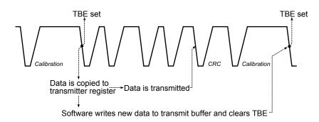
Figure 21-3. Transmit-Buffer Empty driven SENT transfer without Pause Pulse
