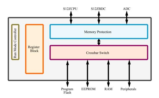
Figure 4-1. S12ZMMC Block Diagram
