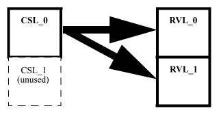
Figure 9-36. CSL Single Buffer Mode — RVL Single Buffer Mode Diagram
