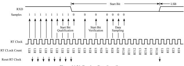
Figure 14-21. Receiver Data Sampling
