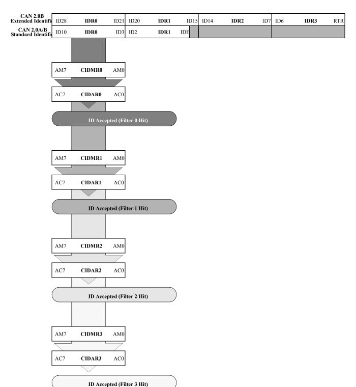
Figure 18-42. 8-bit Maskable Identifier Acceptance Filters
