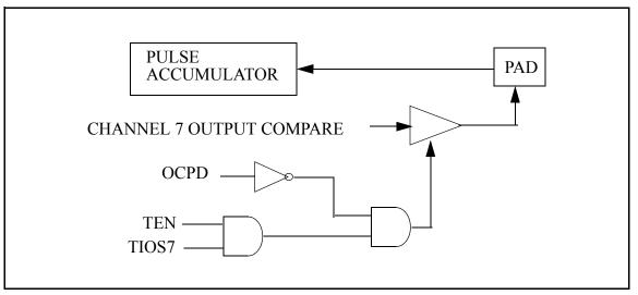
Figure 11-4. Channel 7 Output Compare/Pulse Accumulator Logic
