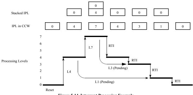
Figure 5-14. Interrupt Processing Example
