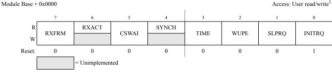
Figure 18-4. MSCAN Control Register 0 (CANCTL0)
