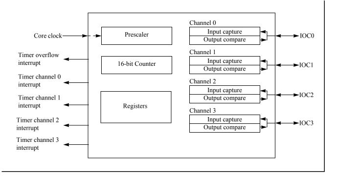
Figure 12-1. TIM16B4CV3 Block Diagram
