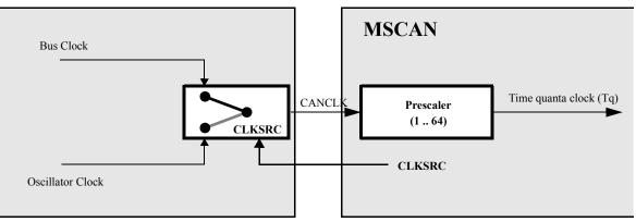
Figure 18-43. MSCAN Clocking Scheme
