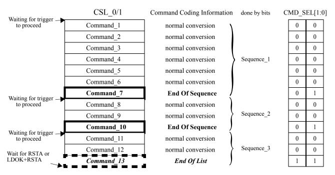
Figure 9-29. Example CSL with sequences and an "End Of List" command type identifier
