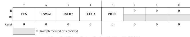
Figure 12-8. Timer System Control Register 1 (TSCR1)
