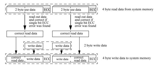
Figure 7-9. 2 byte non-aligned write access
