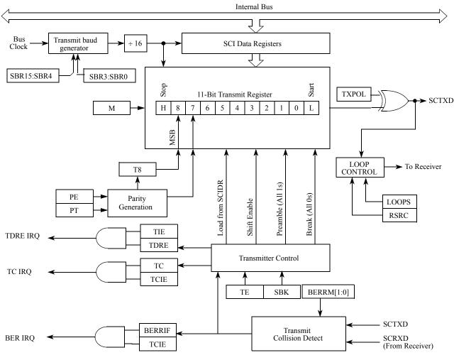
Figure 14-16. Transmitter Block Diagram
