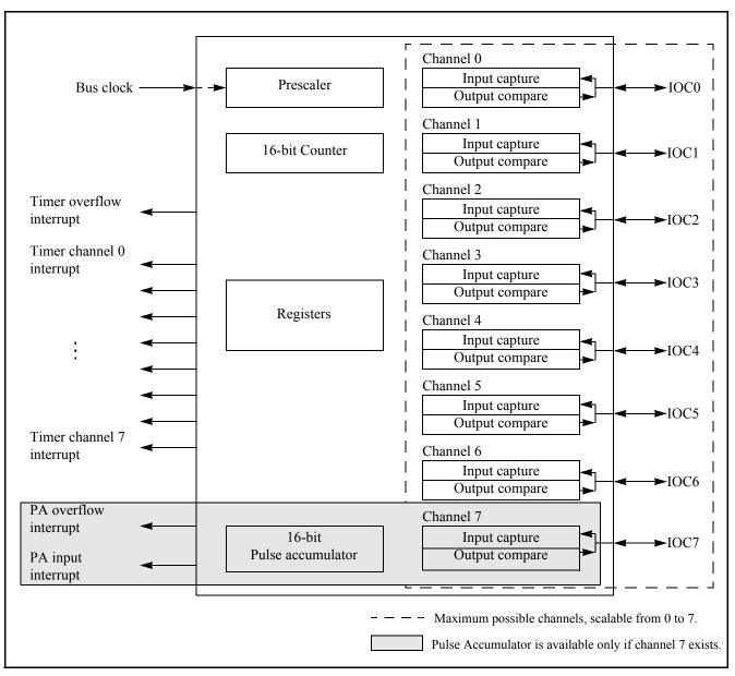
Figure 11-1. TIM16B8CV3 Block Diagram
