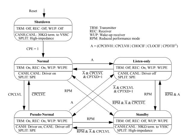
1: A delay after clearing CPDTIF must be accounted for (see description)
