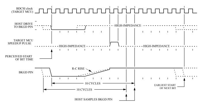
Figure 3-7. BDC Target-to-Host Serial Bit Timing (Logic 1)
