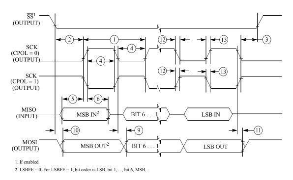
Figure D-2. SPI Master Timing (CPHA=0)
