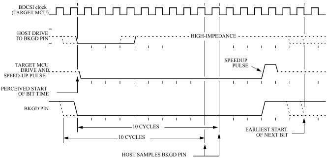
Figure 3-8. BDC Target-to-Host Serial Bit Timing (Logic 0)
