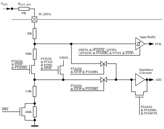
Figure 2-35. HVI Block Diagram
