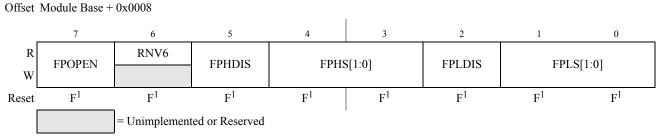
Figure 22-13. Flash Protection Register (FPROT)
