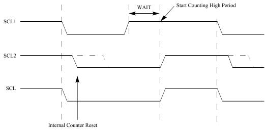
Figure 16-12. IIC-Bus Clock Synchronization
