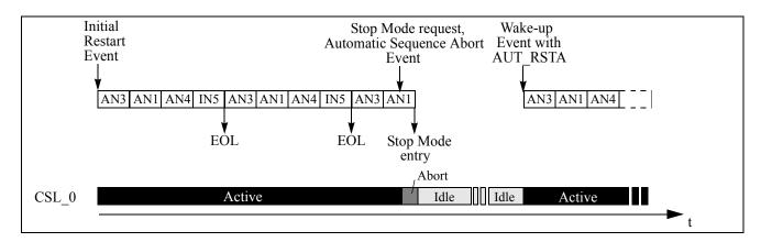
Figure 9-41. Conversion Flow Control Diagram — Continuous Conversion (with Stop Mode)
