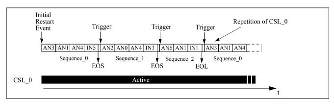
Figure 9-42. Conversion Flow Control Diagram — Triggered Conversion (CSL Repetition)
