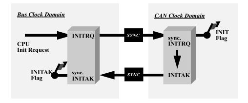
Figure 18-45. Initialization Request/Acknowledge Cycle
