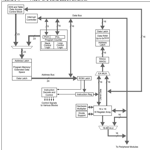
FIGURE 3-1: PIC24F CPU CORE BLOCK DIAGRAM
