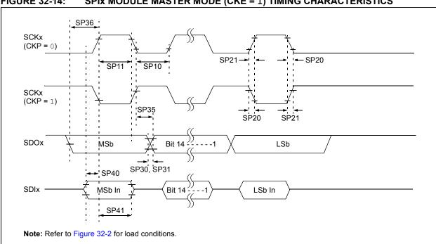
FIGURE 32-14: SPIX MODULE MASTER MODE (CKE = 1) TIMING CHARACTERISTICS
