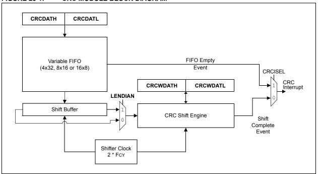
FIGURE 23-2: CRC SHIFT ENGINE DETAIL
