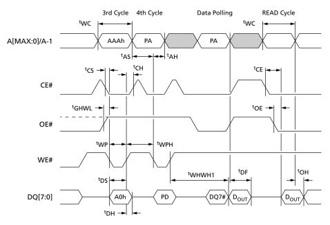
Notes: 1. Only the third and fourth cycles of the PROGRAM command are represented. The PRO-GRAM command is followed by checking of the status register data polling bit and by a READ operation that outputs the data (D<sub>OUT</sub>) programmed by the previous PROGRAM command.
