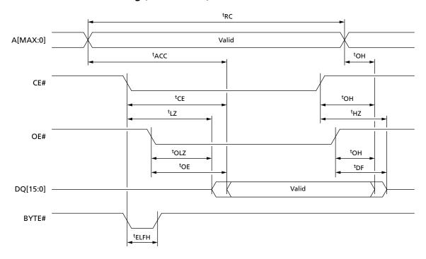
Figure 21: BYTE# Transition Read AC Timing
