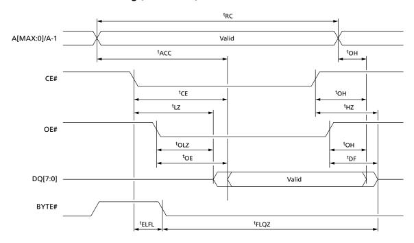
Figure 20: Random Read AC Timing (16-Bit Mode)
