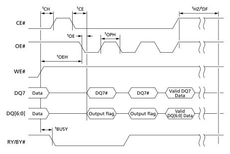
Notes: 1. DQ7 returns a valid data bit when the PROGRAM or ERASE command has completed.
