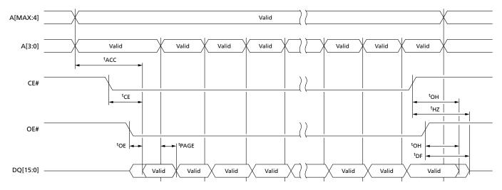
Note: 1. Page size is 8 words (16 bytes) and is addressed by address inputs A[2:0] in x16 bus mode and A[2:0] plus DQ15/A-1 in x8 bus mode.
