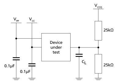
Note: 1. C<sub>L</sub> includes jig capacitance.
