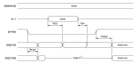
Figure 22: Page Read AC Timing (16-Bit Mode)
