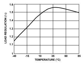
FIGURE 10. LD02 LOAD REGULATION vs TEMPERATURE
