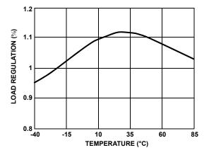
FIGURE 9. LD01 LOAD REGULATION vs TEMPERATURE
