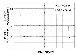
FIGURE 4. LINE TRANSIENT RESPONSE (V<sub>OUT</sub>2)
