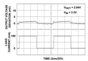
FIGURE 8. LOAD TRANSIENT RESPONSE (V<sub>OUT</sub>3)
