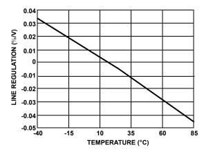
FIGURE 12. LD01 LINE REGULATION vs TEMPERATURE
