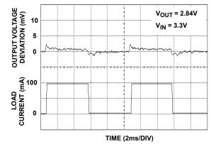
FIGURE 7. LOAD TRANSIENT RESPONSE (V<sub>OUT</sub>2)
