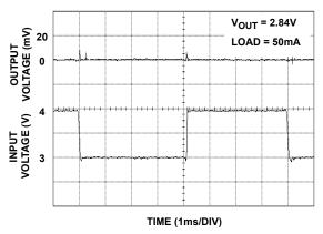
FIGURE 5. LINE TRANSIENT RESPONSE (V<sub>OUT</sub>3)
