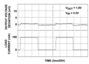
FIGURE 6. LOAD TRANSIENT RESPONSE (V<sub>OUT</sub>1)
