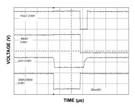
FIGURE 19. SHUTDOWN vs RESET and FAULT
