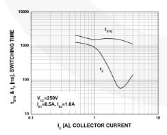
Figure 5. Resistive Load Switching
