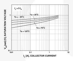
Figure 3. Saturation Voltage
