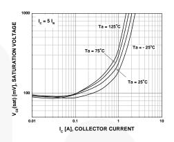
Figure 2. Saturation Voltage
