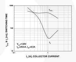
Figure 4. Resistive Load Switching
